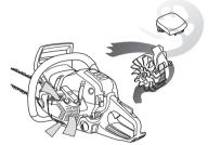
IMPORTANT! In order to maintain operation of the centrifugal cleaning system it must be regularly maintained. Clean the air intake to the starter, the fins on the flywheel, the space around the flywheel, inlet pipe and carburettor compartment.
