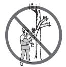
5 You must have a steady stance in order to have full control over the chain saw. Never work standing on a ladder, in a tree or where you do not have firm ground to stand on.
